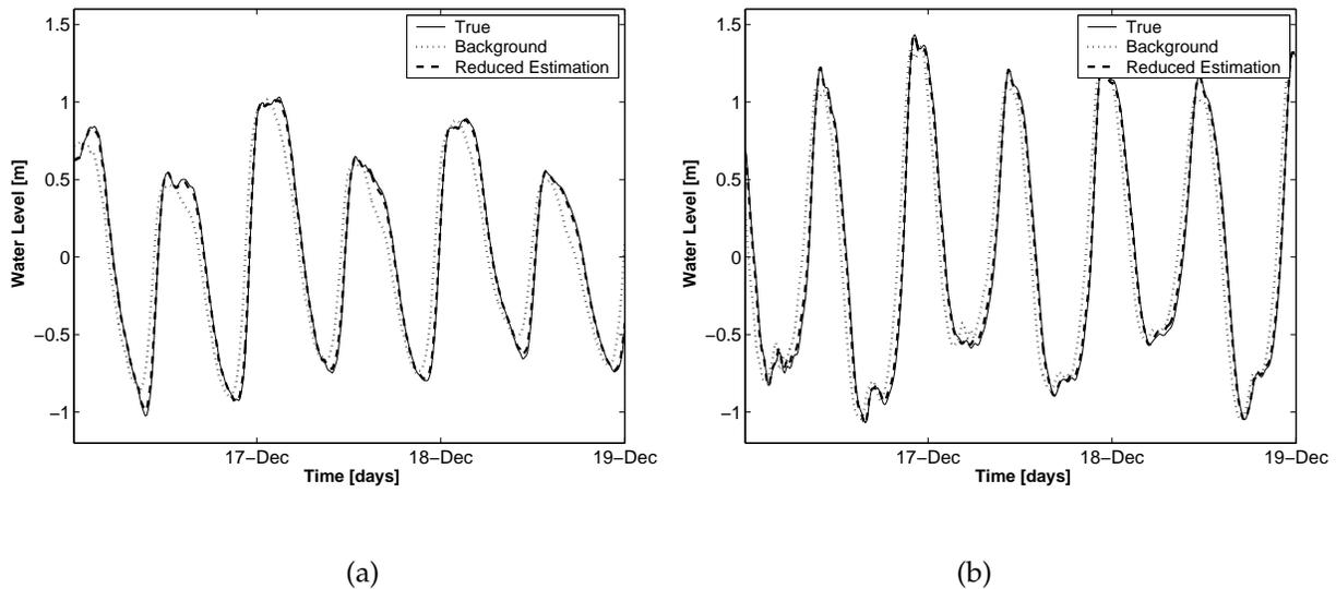
FIGURE 6. Water level timeseries for the period from December 16, 1997, 00:00, to December 18, 1997, 24:00. simulated data (truth), deterministic model without assimilation (background), forecasts with data assimilation after four outer iterations (reduced estimation) at **a)** Den Helder **b)** Hoek van Holland
