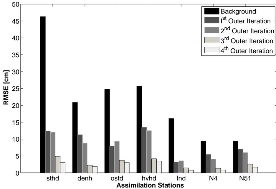
FIGURE 9. RMS errors with respect to water level observations at assimilation stations for calibration over 15 days
