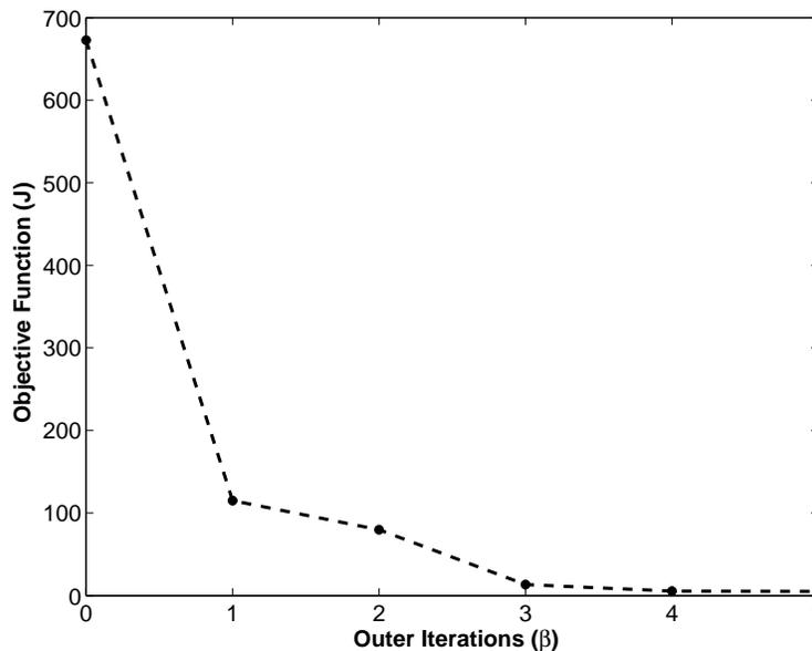
**FIGURE 8.** Graph of the objective function ( $J$ ) versus the number of outer iterations ( $\beta$ ), for the calibration over 15 days
