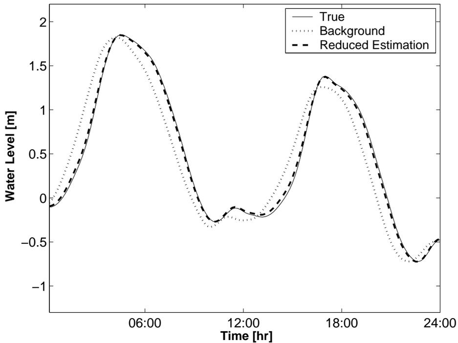
FIGURE 10. Water level timeseries at Hoek van Holland for the period from December 24, 1997, 00:00, to December 24, 1997, 24:00. for simulated data (truth), the initial setting of the calibration parameters (background) and forecasts with data assimilation after four outer iterations (reduced estimation)
