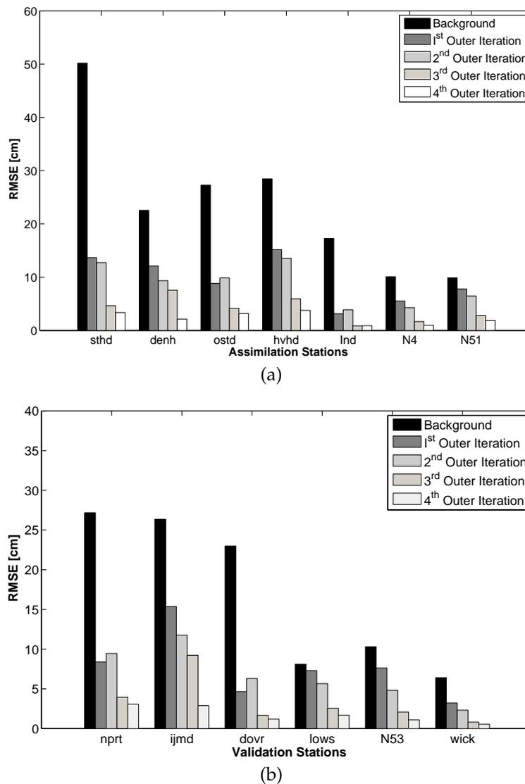
FIGURE 7. RMS errors with respect to water level observations at a) assimilation stations and b) validation stations
