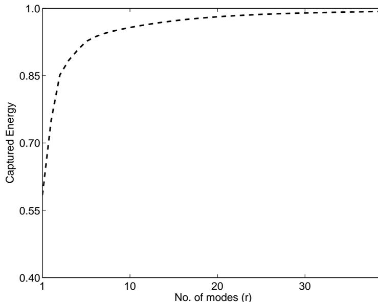
**FIGURE 3.** The POD modes capture energy for an ensemble of 210 snapshots of the water-level  $h$ (m), velocities  $u$  and  $v$
