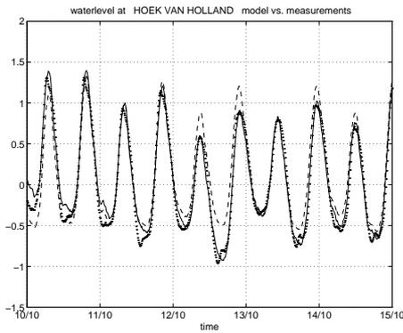
figure 3: Waterlevels with astronomic (dashed) and corrected (line) boundary conditions vs. measurements (dotted)
