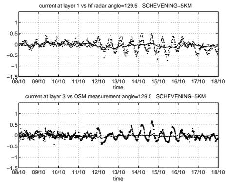
figure 4: Cross-shore currents for algebraic (line) and  $k - \varepsilon$  model (dashed) vs. measurements (dotted)
