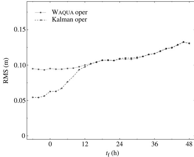
Figure 5. Operational evaluation for location Scheveningen. RMS errors for different forecast ranges with and without Kalman filter.
