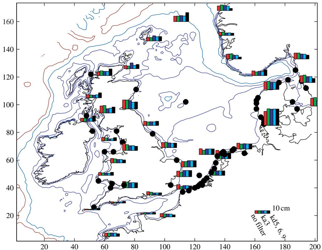
Figure 6. Impact of various Kalman filter configurations on RMSE: RMSE for forecasts from 00.00 to 06.00 on 11 November 1999. DCSM version 5 without a filter and with ka3, kd5, kd6 and kd9 filters.
